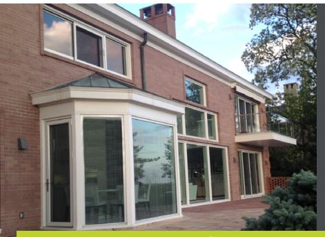
Solar manufactured 29 windows, 6 vertical wall systems, 2 inswing terrace doors, 2 outswing single doors, 3 sliding glass doors, and 1 sliding glass window for this complete glazing package. The project features Solar's standard White Duracron frame finish and LoE 272 insulated glazing. Consistent sight lines provide the home's facade with a cohesive appearance.
