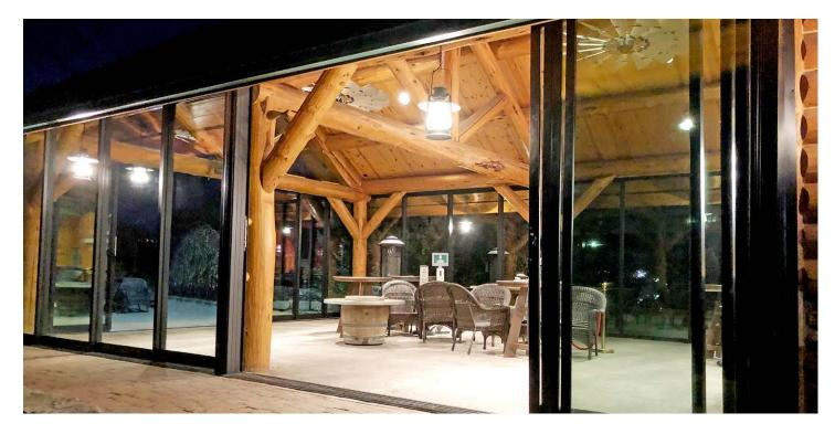
lake. All of the units are over 9 ft. in height and allow guests to enjoy the scenery through floor-to-ceiling glass. An ADA-compliant, thermally-enhanced sill was chosen for ease of access for handicapped guests and to assist in regulating internal temperatures. To further assist in protecting guests, one-inch insulated glass was utilized on all units.
