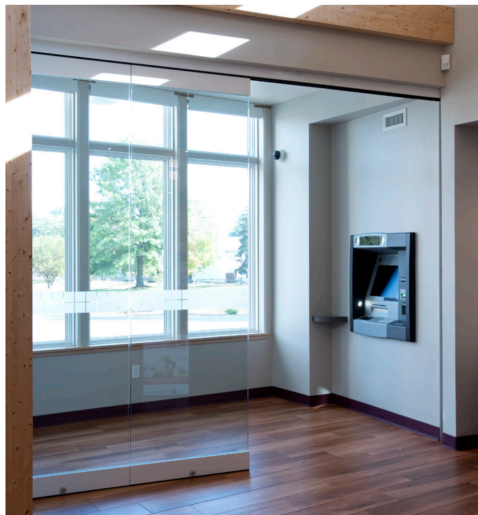
CLEAR GLASS WALL WITH NO FLOOR TRACK
