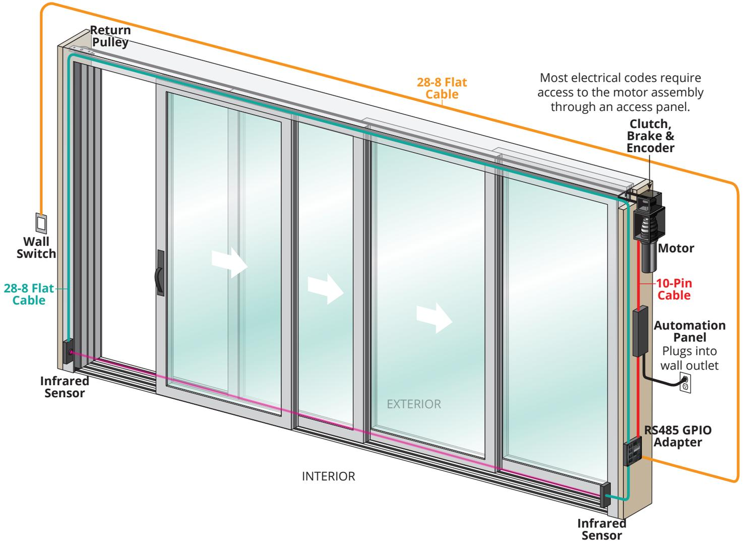
Most electrical codes require access to the motor assembly through an access panel.
