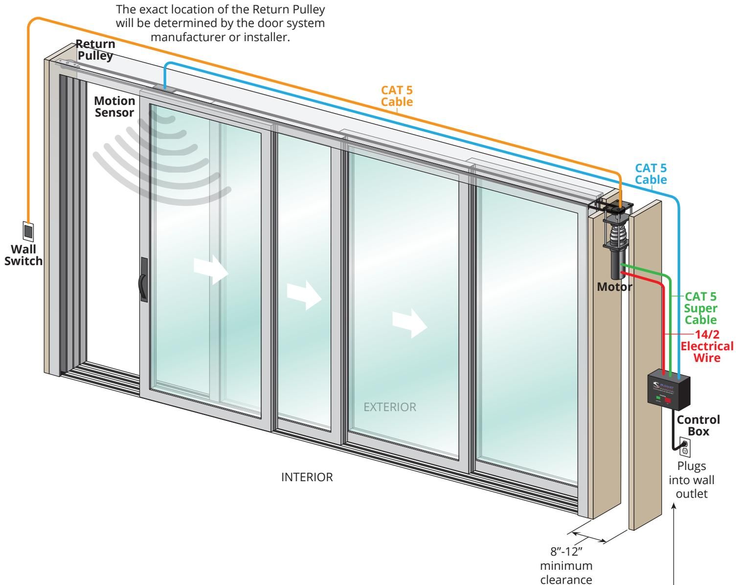
Recommended location for Control Box is in a mechanical closet at chest height plugged into its own dedicated 100V 15 amp outlet within 100 feet of Motor.
