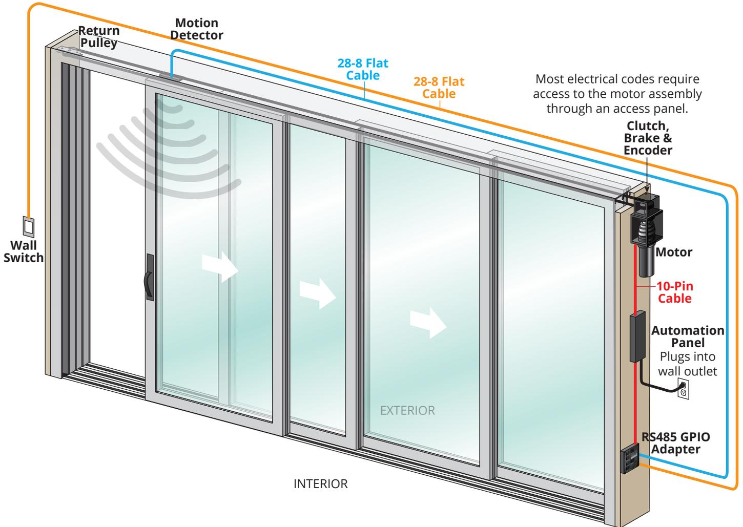
Most electrical codes require access to the motor assembly through an access panel.
